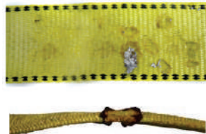
Sling Weld Splatters and Charring/Melting
